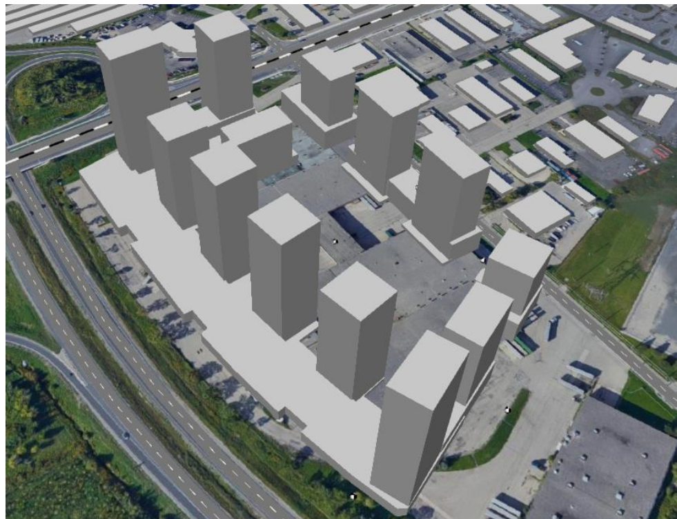
Figure 2: Project massing for Phase 2 as included in the CadnaA noise model.
