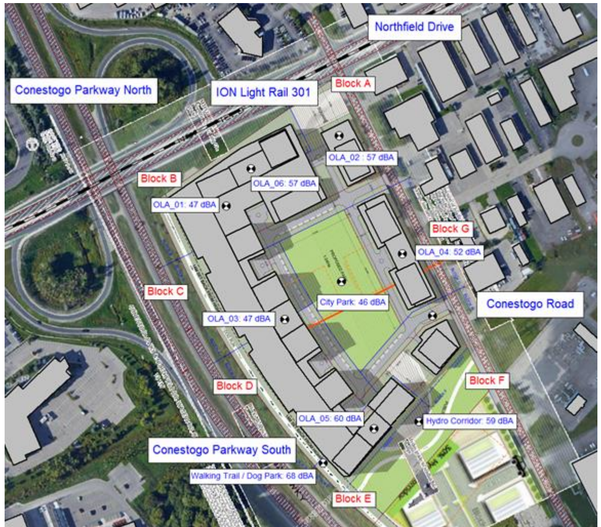
Figure 4: Final Phase OLA Predicted Sound Levels, Road and Rail
