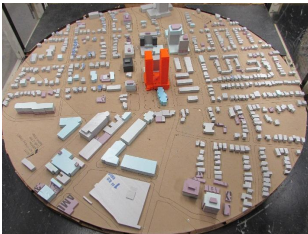
Image 3B: Wind Tunnel Model of the Proposed + Existing Surrounding Buildings
