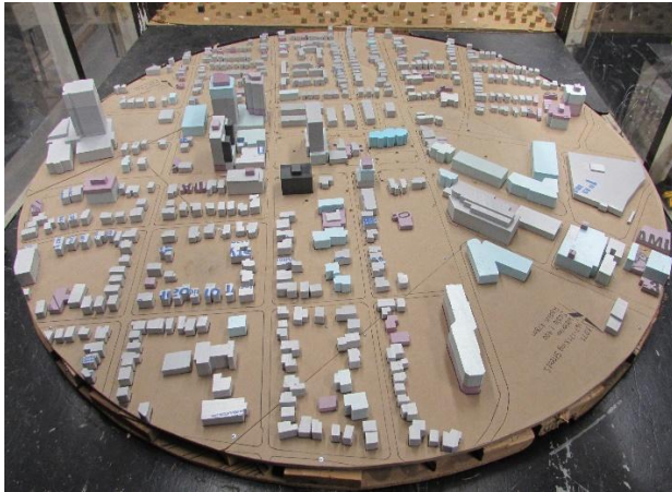
Image 3A: Wind Tunnel Model of the Site and Existing Surrounding Buildings
