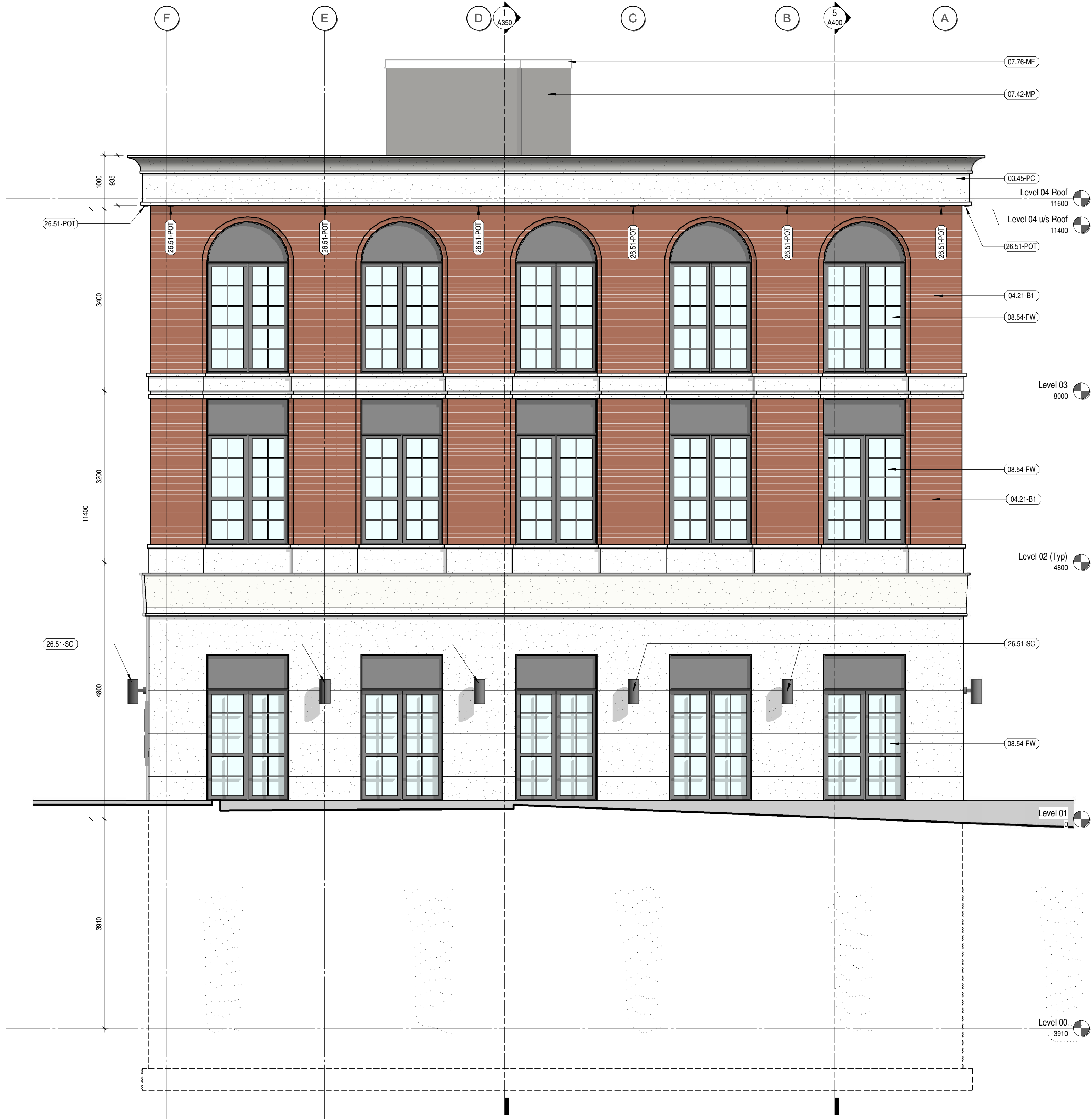
2 East Building Elevation - Rear Yard 1:50
