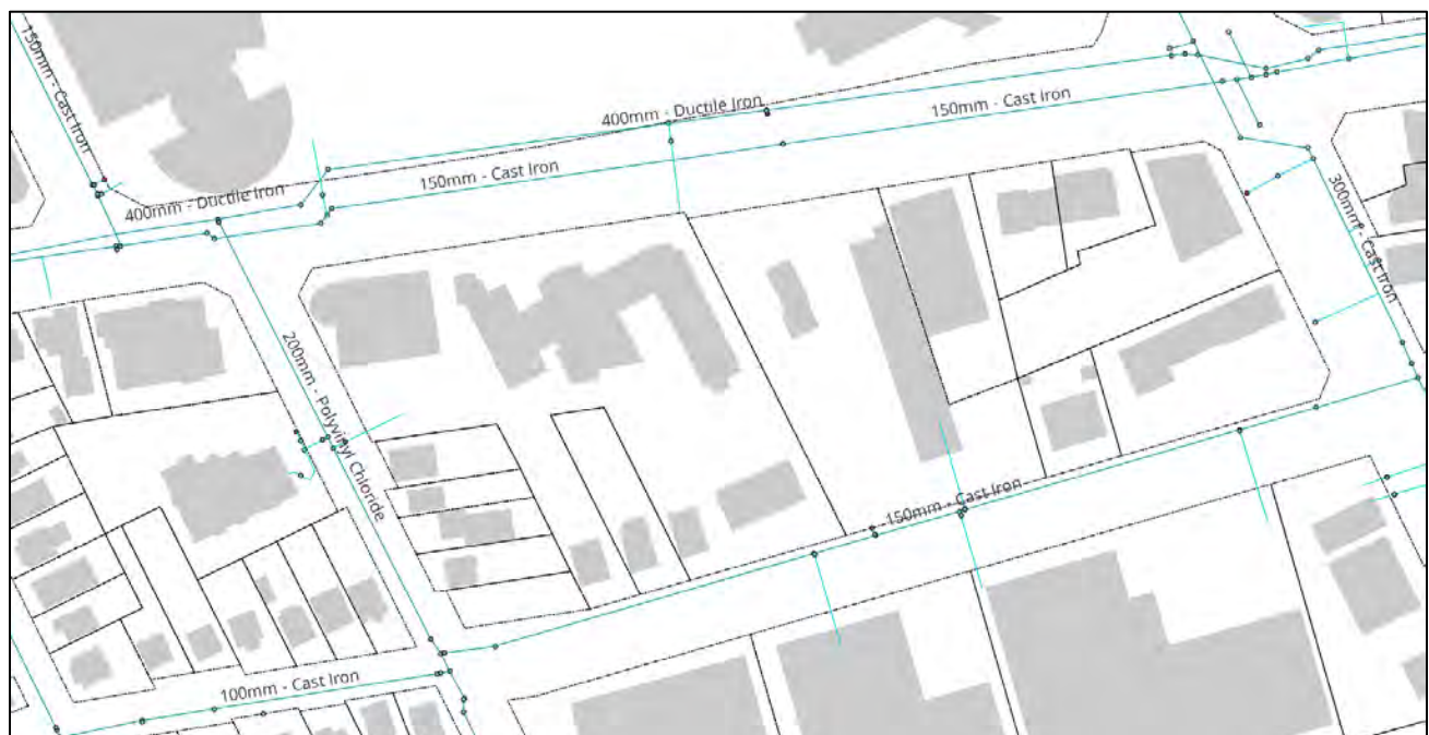
Figure 1: Existing Water Servicing
