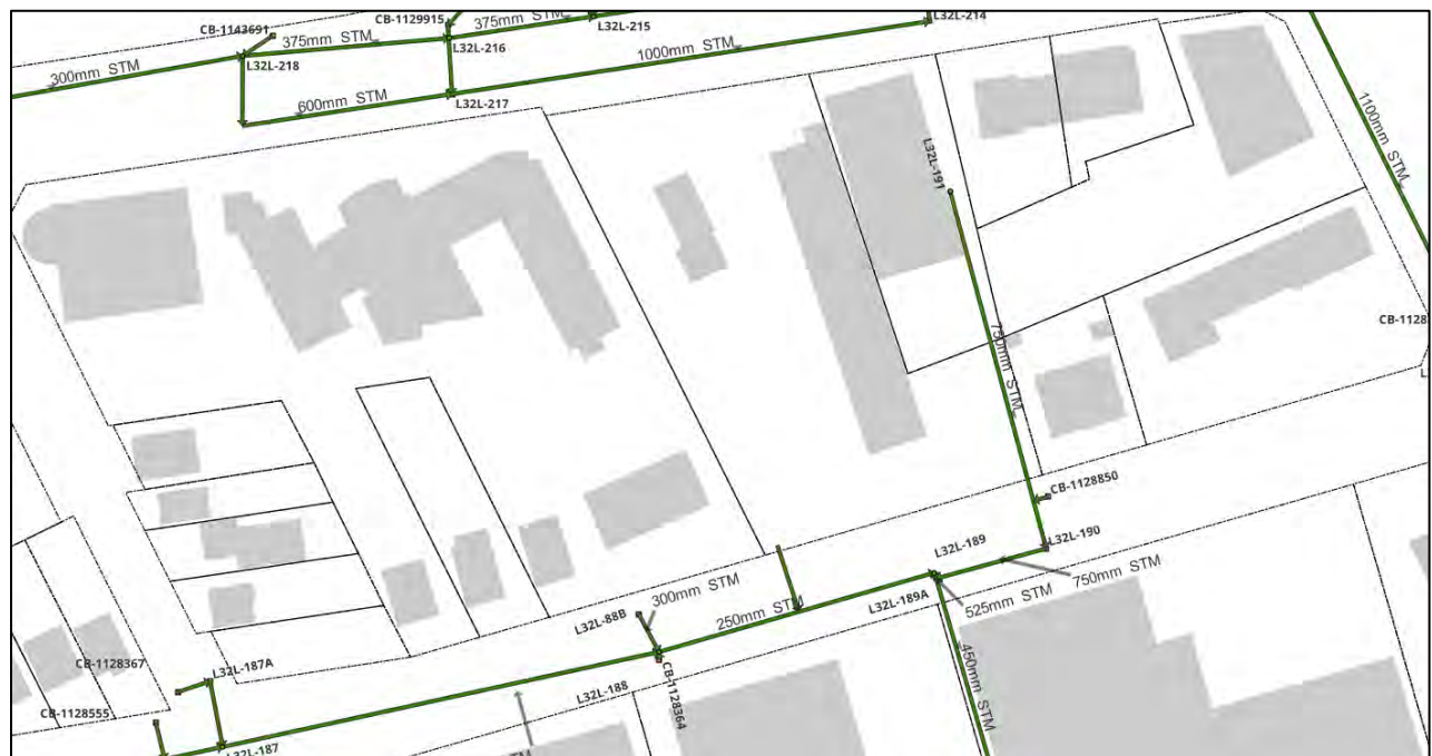
Figure 3: Existing Storm Servicing
