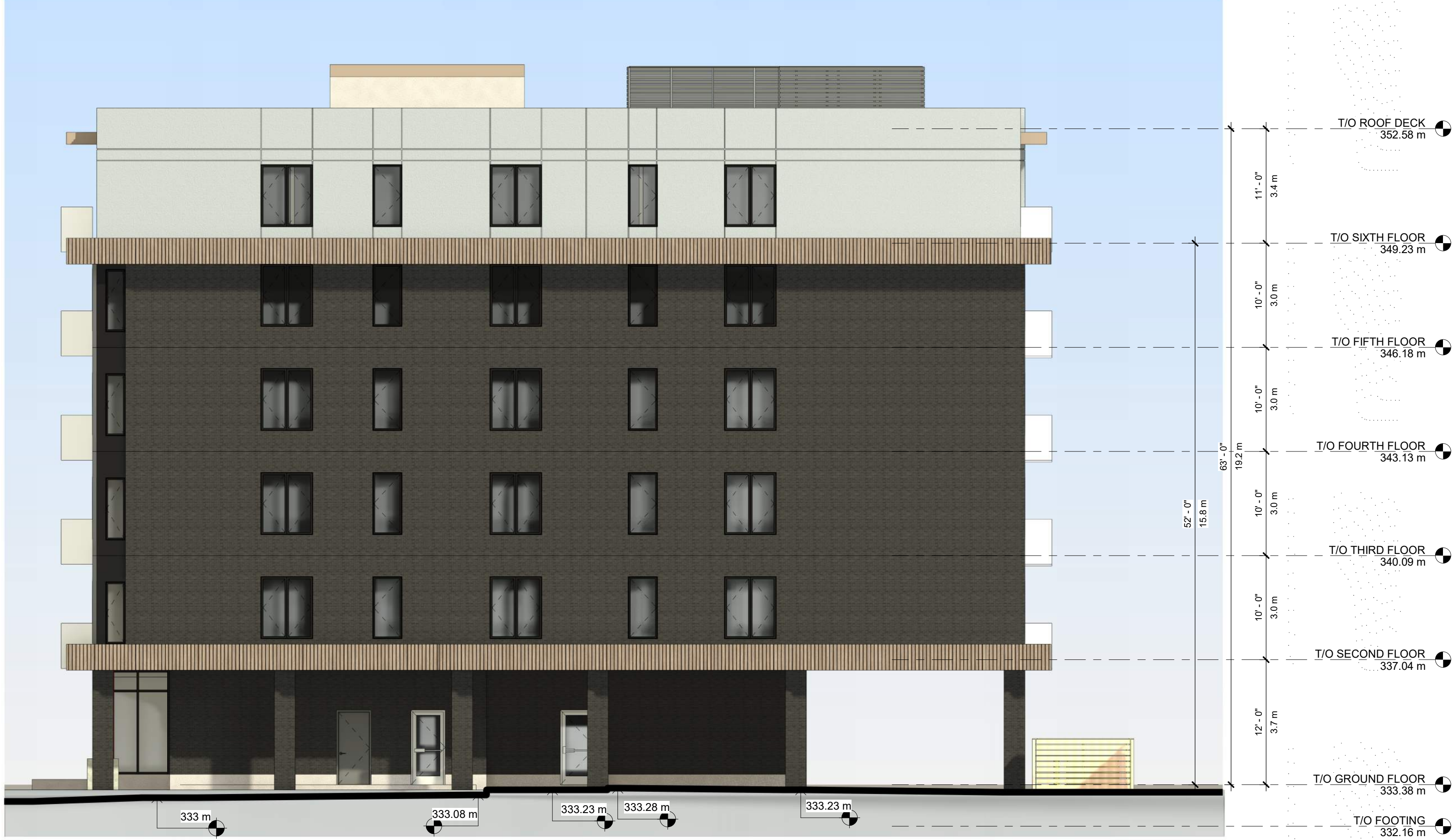
2 SD-NORTH ELEVATION ASP-300 1/8" = 1'-0"
