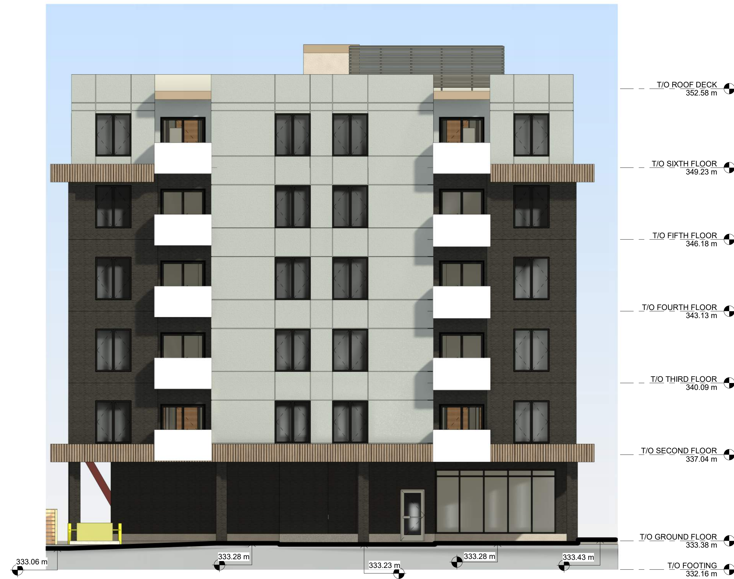
4 SD-WEST ELEVATION ASP-300 1/8" = 1'-0"
