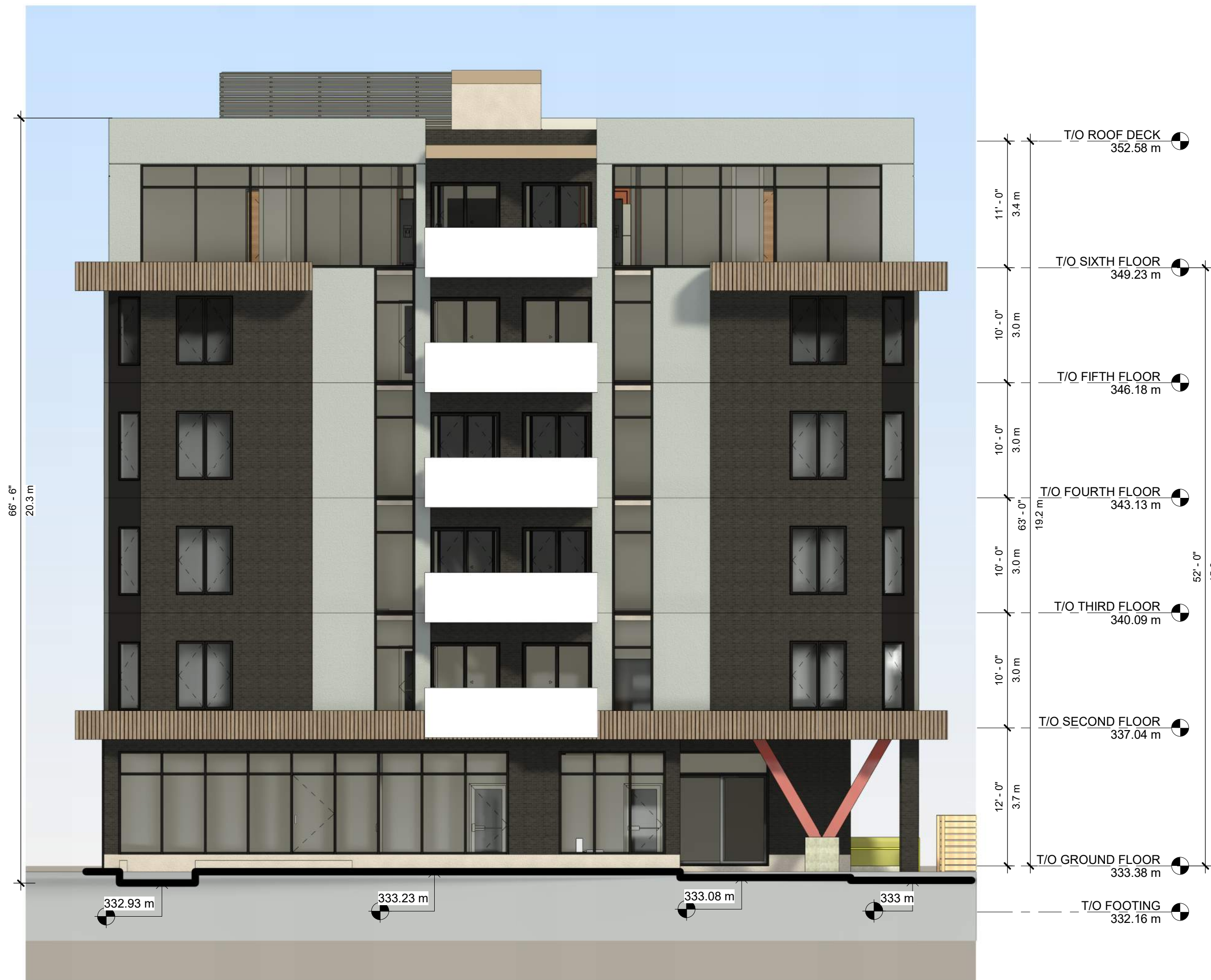
3 SD-EAST ELEVATION ASP-300 1/8" = 1'-0"
