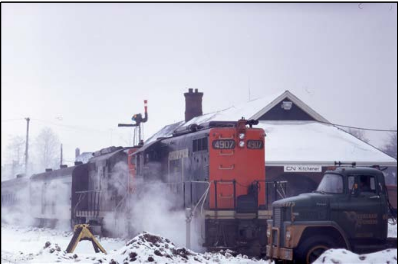
Remembering February of 1971 when CNR – GTW cross border passenger train The Maple Leaf, No. 159 from Toronto to Chicago on its daily 0950 hours stop at the CNR station in Kitchener. This cold winter day reminds us that passenger trains were heated by steam heat by way of steam generators on diesel powered trains. These 2 photos show a red board on the train order semaphore for 159, the old baggage cart on the platform and a classic old Dodge truck for Overland Express.
